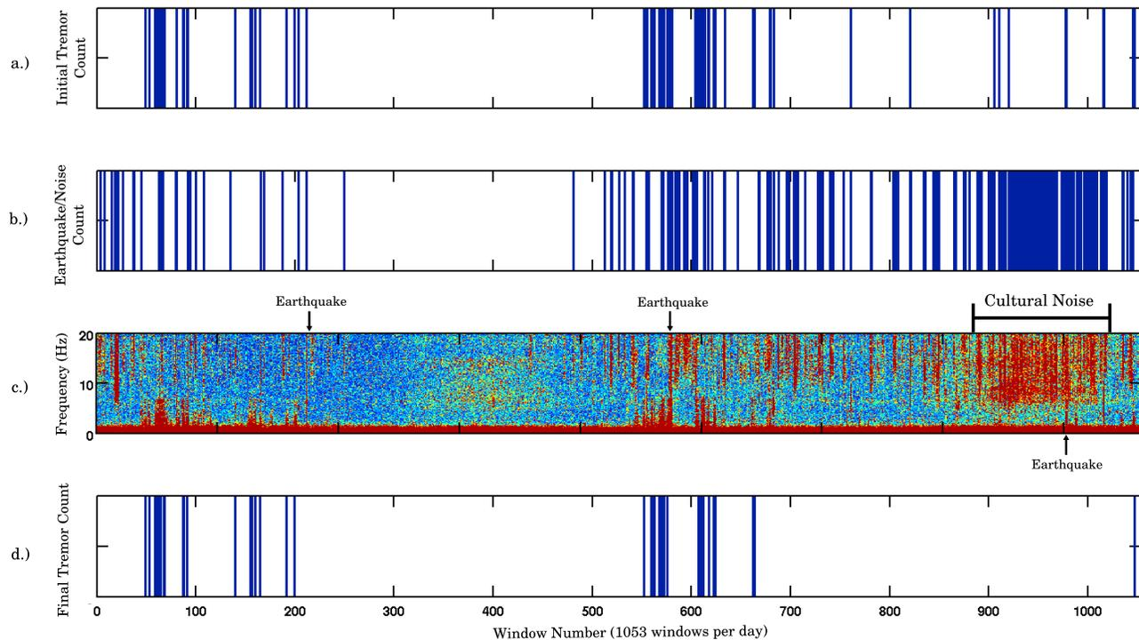
**Figure 2.** Illustration of the spectral detection method for one day (2008 JD 215) showing (a) initial tremor detections, (b) earthquake and cultural noise detections, (c) the daily stacked network-wide spectrogram with the color axis saturated at the detection threshold (red), and (d) final tremor detections determined by subtracting Figure 2b from Figure 2a. The high level of cultural noise and several earthquakes are indicated on the spectrogram.
